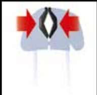
IN NERO, DISPOSITIVO BREVETTATO PER TUBI DI PICCOLO DIAMETRO IN BLACK, CLOSE-UP PATENTED OF CLAMP JAW REDUCER CLOSE UP OF CLAMP
